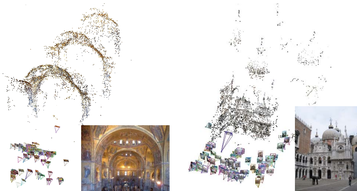
Fig. 14 Additional models reconstructed from the San Marco Square dataset. Left: the nave of the church (81 cameras). Right: the side of the church (90 cameras).
