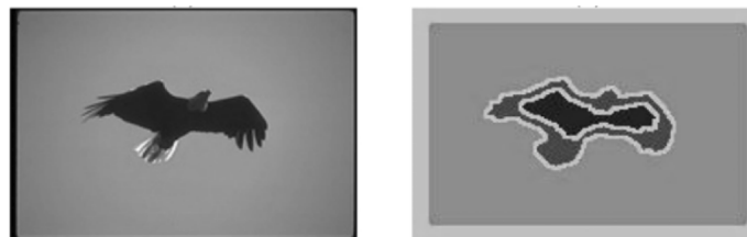
Figure 3. Demonstration of the "contour-as-a-texture" problem using a real image. (a) Original image of a bald eagle. (b) The groups found by an EM-based algorithm (Belongie et al., 1998).
